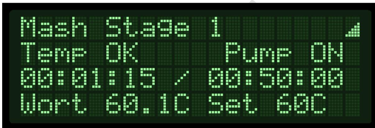
As before the elapsed/total time for this stage and the estimated Time Left for the entire brew will be displayed on a rotational basis on the 3<sup>rd</sup> line.
