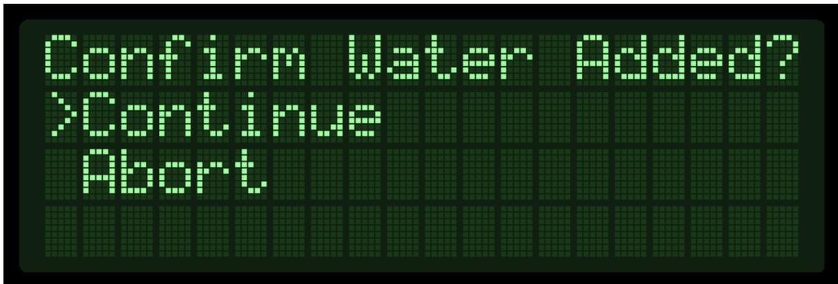
EINBREW will automatically begin a Pump Ventilation cycle to ensure that the water is brought through the system properly with no trapped air. No user intervention is required.
