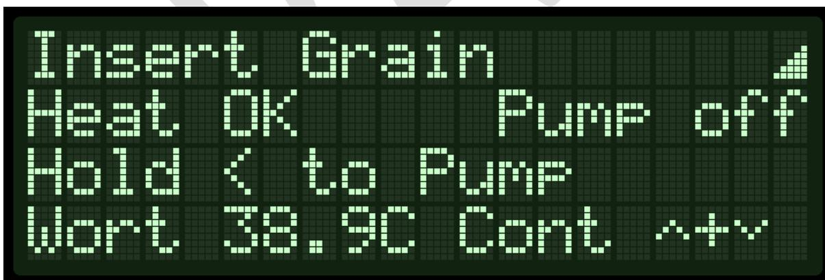
When inserting the vessel and stirring in the grain, you can also optionally press and hold the ◀ button to pump in water. As a safety feature, the pump will only activate when the button is held. Ensure that you do not allow the water level to flow over the top of the inner vessel and let grain enter the system – you want to minimise this to ensure the wort is free of debris when mashing.
