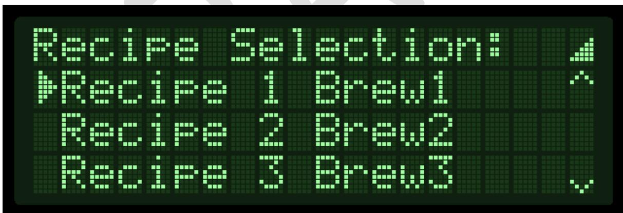
Once you've selected a Recipe, you can review (and change) its settings. Select a Recipe parameter using the ▲ ▼ buttons, then use the ◀ ▶ buttons to alter the value. To abort the process, select the **Back** option to return to the Main Menu.
