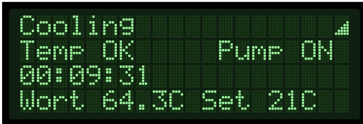
First you must wait for the wort temperature to drop below the Pump Max Run Temp, normally 95C, this should take around 5 to 10 minutes, once the pump starts circulating the wort, you can turn on the coolant flow to the rear of the EINBREW, the wort temperature will start to drop rapidly. Cooling of around 30 litres from 95C to 24C will take just around 25 minutes, depending on coolant water temperature. **We strongly recommend that you always save your exhaust water.**
