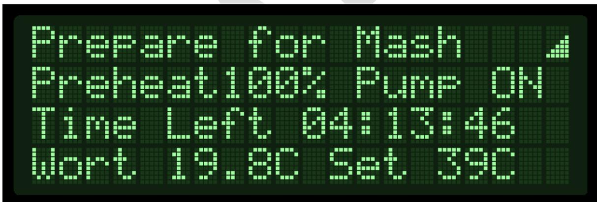
Whilst the water is preheating, the Handheld will display the heating status, the pump status and the current Wort temperature versus the Set (desired) temperature. The 3<sup>rd</sup> line of the display will also display on rotation the estimated total brew time left (Time Left), and the current stage runtime versus the estimated total time at present heating rate (e.g. 00:04:15/00:18:04). All times are in Hours, Minutes and Seconds (hh:mm:ss).
