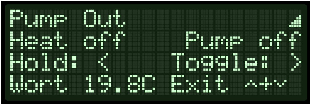
To activate the pump, press and hold the ◀ button. As a safety feature, the pump will only activate when the button is held. If you need to activate the pump for a longer period, you can toggle it on and off with the ▶ button. Once you've finished pumping out, press the ▲ and ▼ buttons together to exit the **Pump Out** mode and return to Standby.
