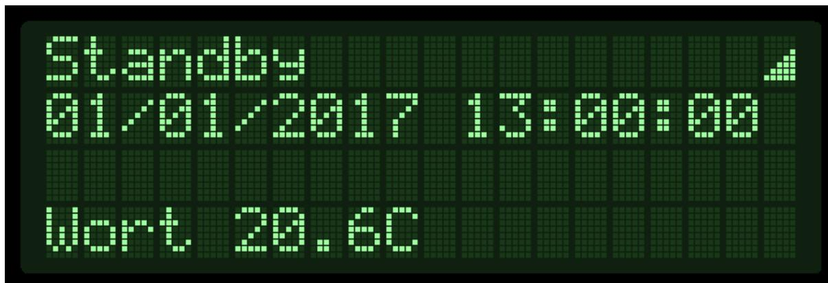
When EINBREW is not in use, the display will indicate that it is in Standby mode, along with the present Date and Time. The “signal” icon at the top-right of the display indicates that the Handheld controller is connected to the EINBREW system successfully. The temperature of the main vessel is indicated at the bottom as the Wort temperature.
