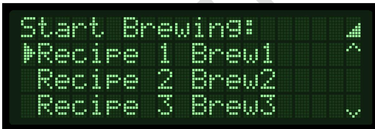
Once you've selected a Recipe, you can review (and change) its settings. Select a Recipe parameter using the ▲▼ buttons, then use the ◀▶ buttons to alter the value. See the **Recipe Menu** section for more details. To abort the process, select the **Back** option to return to the Main Menu.
