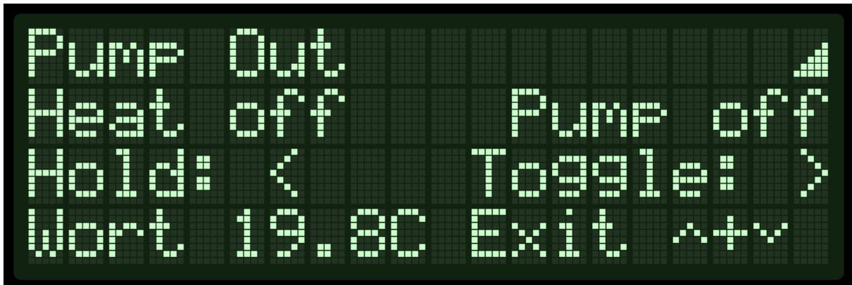
To activate the pump, press and hold the ◀ button. As a safety feature, the pump will only activate when the button is held. **If you need to activate the pump for a longer period, you can toggle it on or off** with the ▶ button. Once you've finished pumping out, press the ▲ and ▼ buttons together to exit the **Pump Out** mode and return to Standby.
